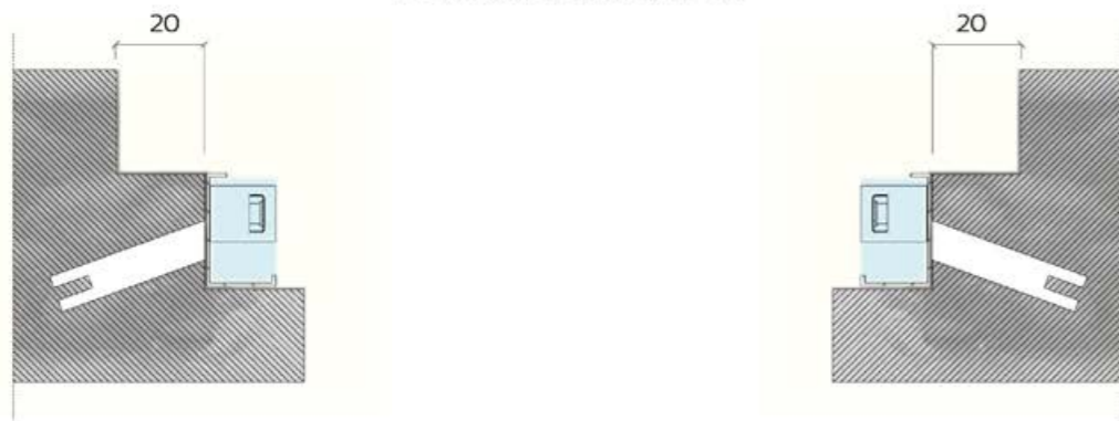
montaggio a centro muro assemblage in the middle of the wall
